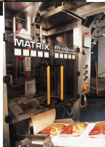
The Matrix ProStar VFFS bagger places the desired weight of sliced apples into pillow-shaped plastic bags made from special MAP film.
